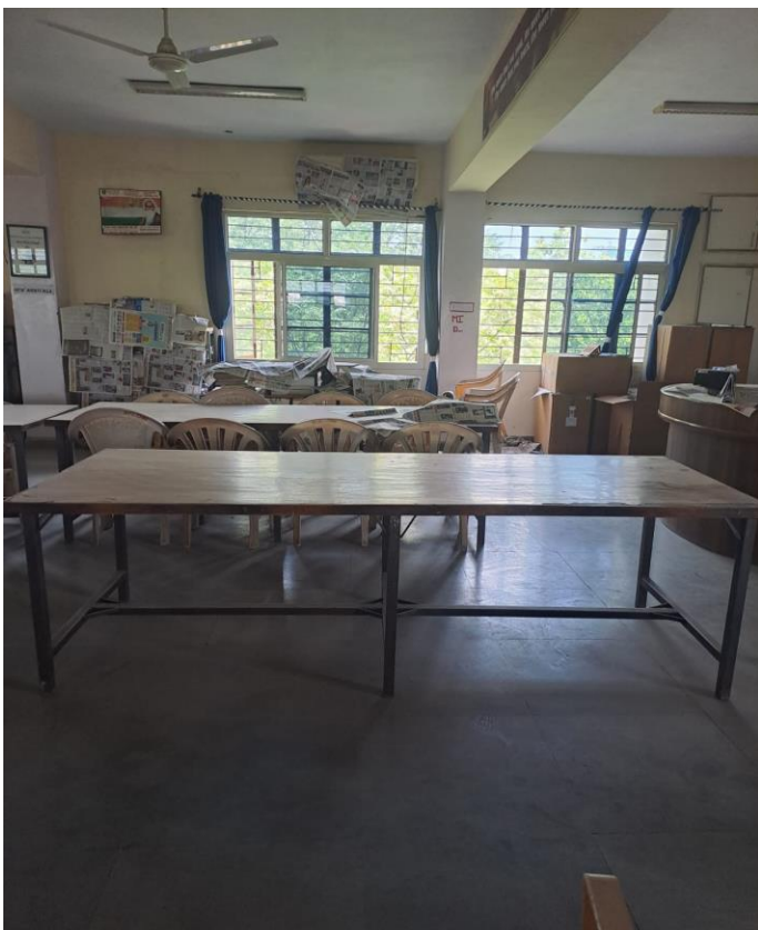
Library Tables 8' x 3' with Iron angle frame (l) L x b x h = 7'10" x 2' 7" x 2'5"
