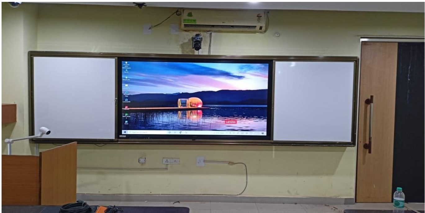
Interactive Flat panel 85'' with shutter (after closing shutter to be use as white board)
